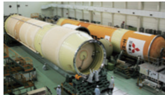
Assembly of an H-IIA launch vehicle The manufacturing of parts of a launch vehicle involves more than 350 primary subcontractors, and the number increases to more than 1,000 if every subcontractors are included. "This may not be rewarding from a commercial perspective because sophisticated technologies are required to manufacture and to finish the products as designed, and because the number of orders is small. Still, the subcontractors support us saying that they can expand the production area by obtaining sophisticated technologies," said by Mr. Nimura.
